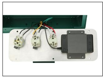
Figure 73. Control panel wiring.
